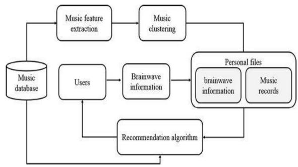
This block diagram illustrates the workflow of Mindsymphony's system. The breakdown of its components is as follows:
