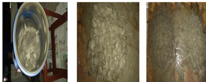
Mixing process of ECC and Conventional Concrete
