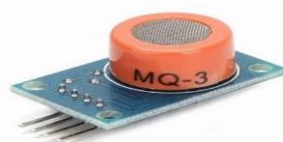
Fig 2:- MQ-3 sensor with crash board
