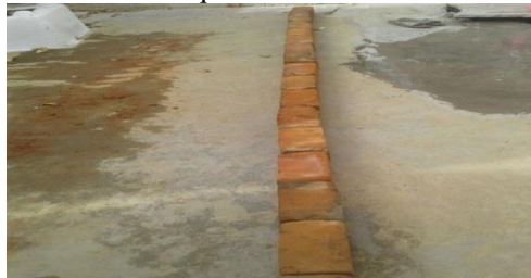
Fig. 6: Dimensions tolerance test
