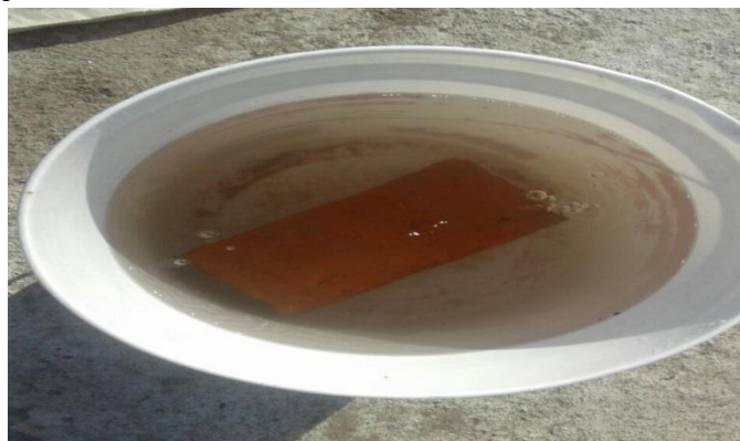
Fig. 4: Water Absorption test
