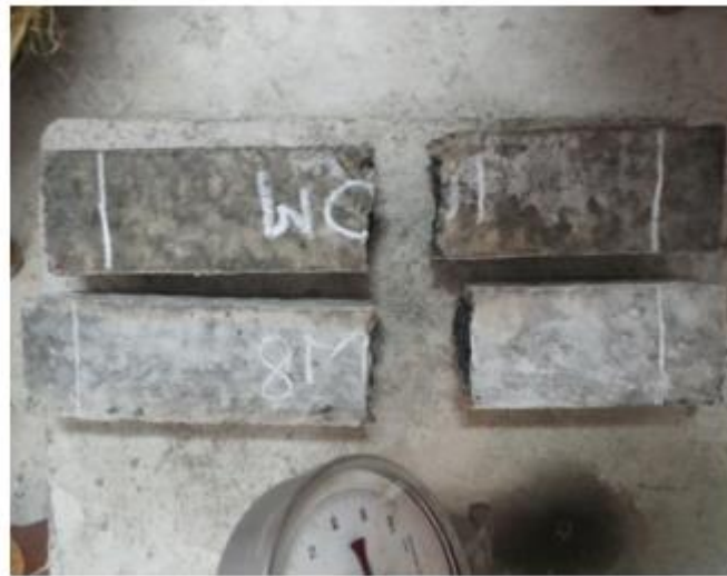
Fig -9 beam failure pattern
