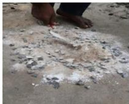
Fig -1 Geopolymer concrete dry mix
