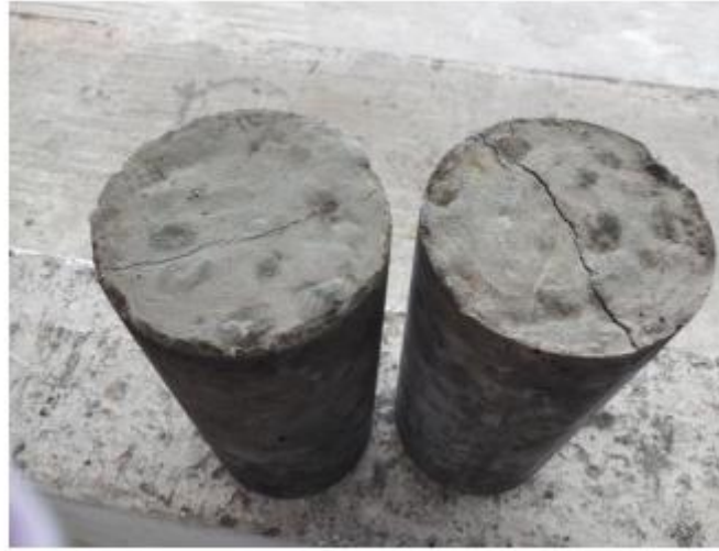
Fig -8 cylinder failure pattern
