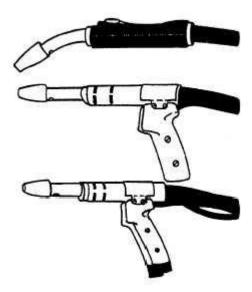
In GMA welding guns as Shown in the figure when using these guns, the wire is fed to the torch by an automatic wire feeding machine which pushes the wire through a flexible tube to the arc point.
