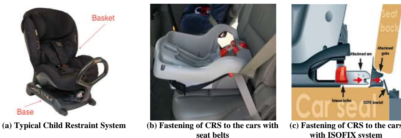
Fig. 2: Child restraint systems & its fastening to cars
