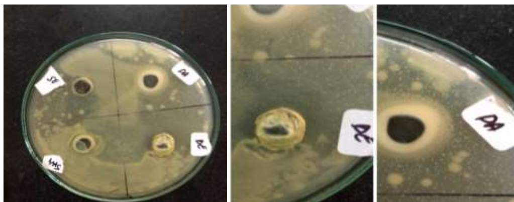
Fig. 4: Antibiotic susceptibility test of different hand wash product (Dettol hand wash, Dettol sanitizer, and Patanjali)
