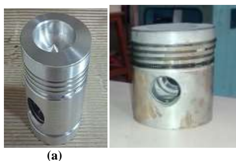
Fig. 8: (a) Uncoated piston (b) Zirconia Coated Piston
