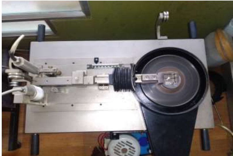
Fig. 1: Pin-on-disc sliding wear testing machine with integrated system
