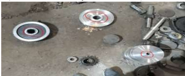
Fig. 1: Spur gear with under sized hole
