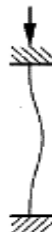
Fig. 5: End columns taking a complete load of upper frames and lower frames
