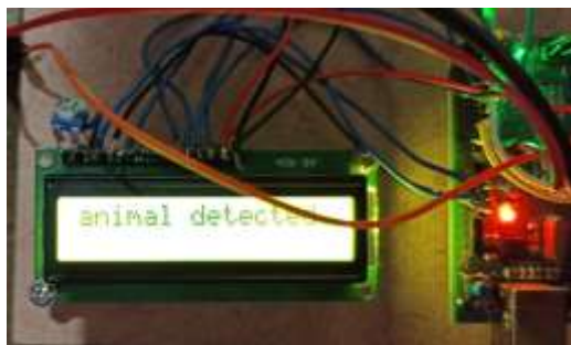
Fig 6.3. Intimation through LCD display
